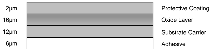
Tape Construction - Typical Thickness
